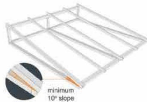
**Step 2** Install Alderon RS with corrosive resistant bolt and weather resistant seal.
