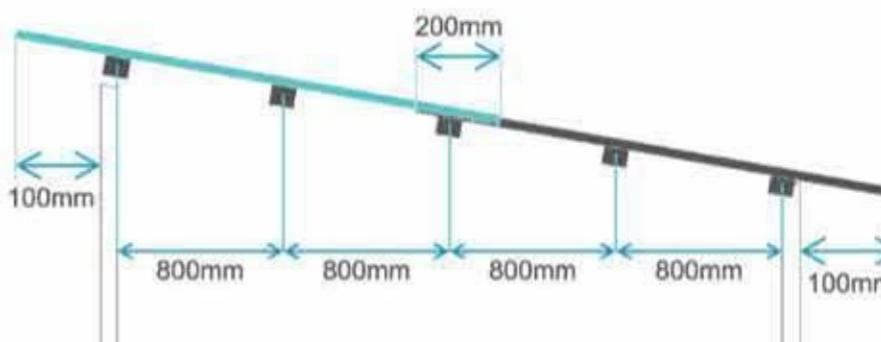
**Step 4** Install Alderon RS with corrosive resistant bolt and weather resistant seal.
